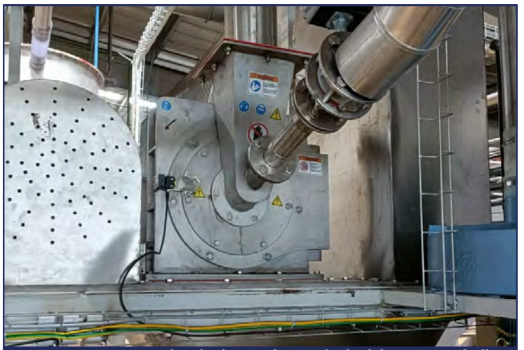
DP@ UNV-320PD-EX [explosion-resistant design] for sugar grinding
