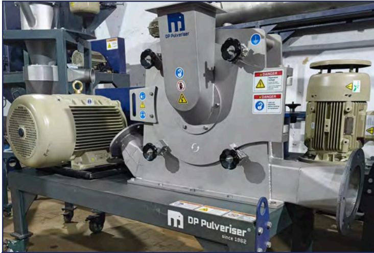
DP@ UNV-320BT for grinding of tea-fibre
