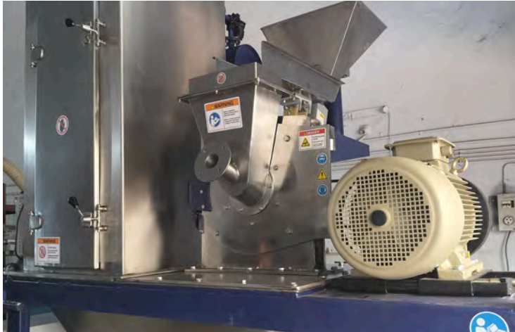
DP@ UNV-320PD for grinding of potato flakes before dispatch
