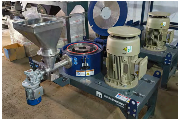
DP@ ACM-15 for pigment grinding before dispatch
