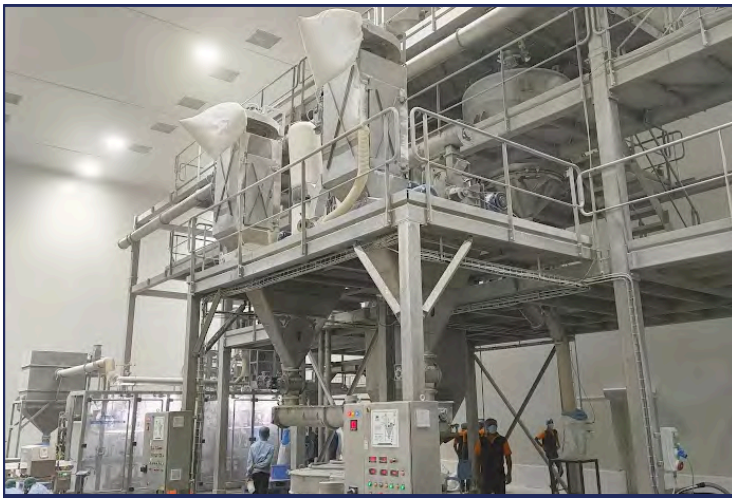
2 Nos. DP@ CNT-320 CONTRA Pin Mill for potato flakes grinding
