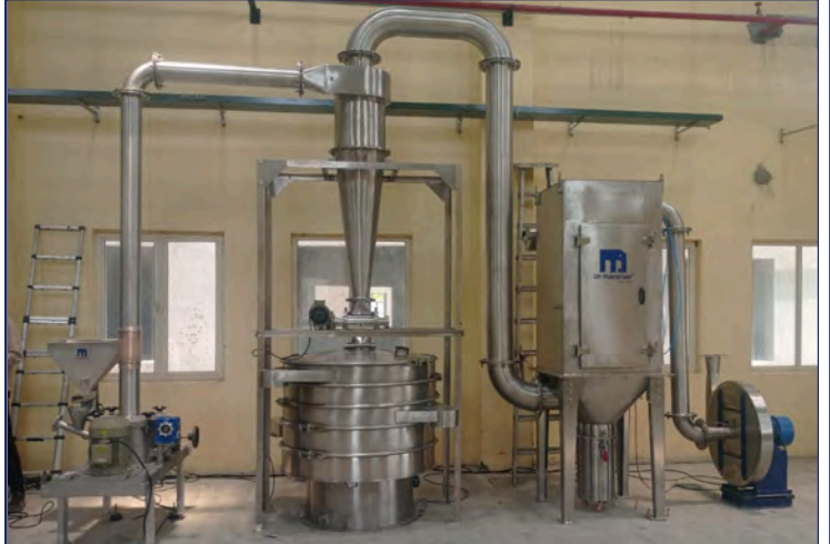
DP@ ACM-15 system installed at BPCL, Delhi for biomass grinding
