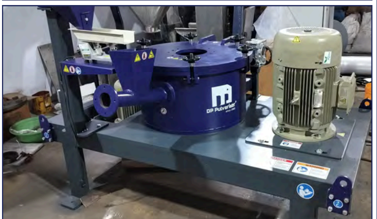
DP@ ACM-30 for grinding of synthetic graphite
