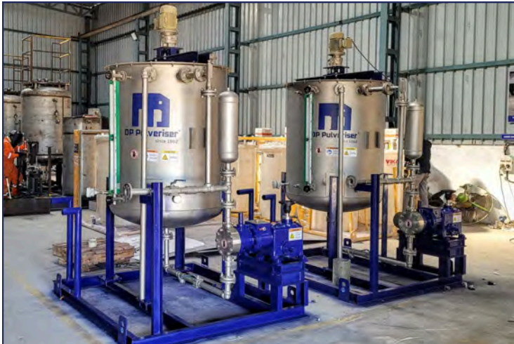
DP@ Liquid Dosing Tank system ready to ship to the middle-east
