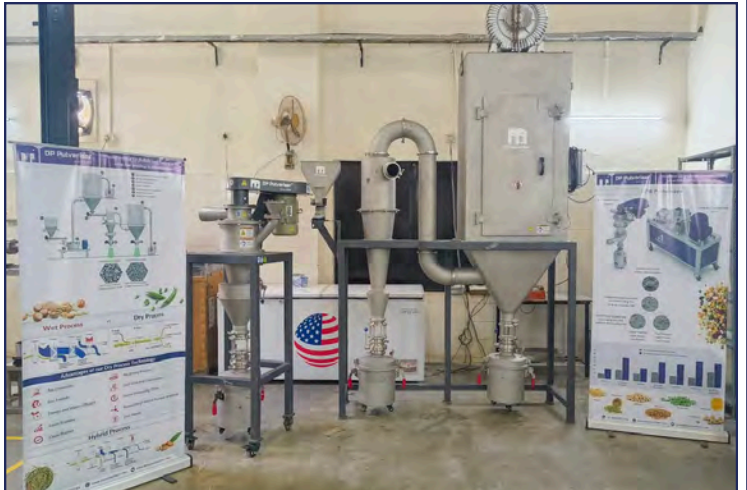
DP@ ARV-120 AEROVA for dry protein shifting application
