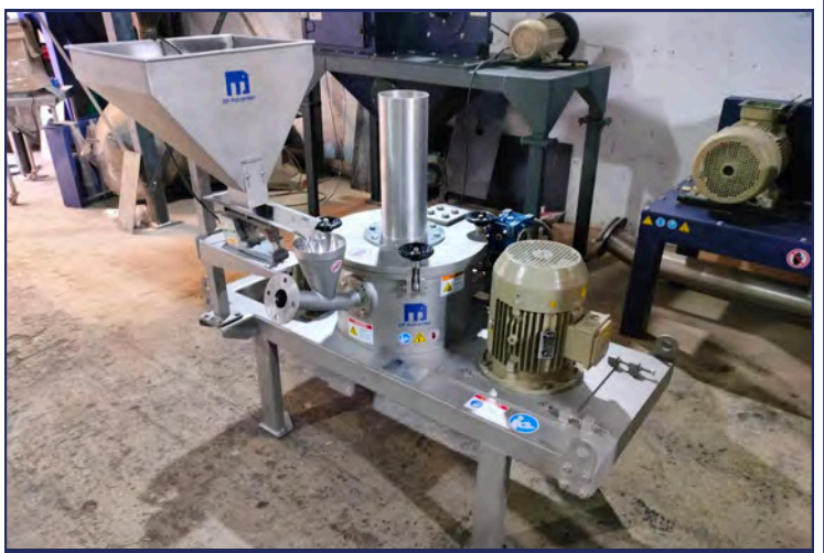
DP@ ACM-10 in SS304 contact and non-contact parts
